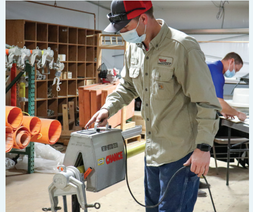
Cody Ellis, journeyman lineman, runs a hot stick tester along the length of a layout arm at the Scott City warehouse with the assistance of Quinten Wheeler, manager of safety and compliance.
